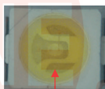
Sulfide materials, stent Bowl Cup silver layer black 硫化后支架碗杯银层变黑
